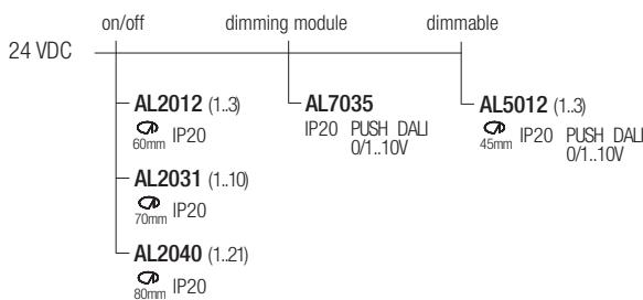
Note: dimming module AL7035 to be used in combination with a 24VDC power supply
