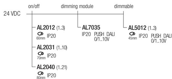
**Note:** dimming module AL7035 to be used in combination with a 24VDC power supply
