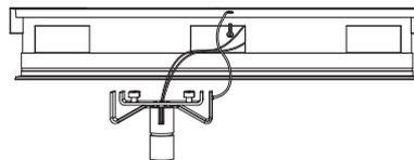
Insert the light module into the structure and position it. The module attaches magnetically.
