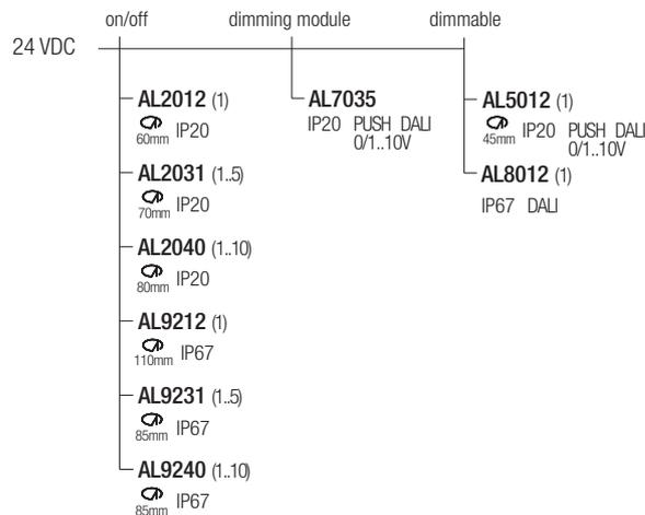
Note: dimming module AL7035 to be used in combination with a 24VDC power supply
